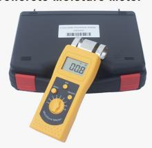
DM200 Concrete water testing instrument adopted the high frequency principle based on the introduction of the most advanced technology from foreign country. In other words, there is a fixed frequency inside the equipment Once the moisture of the detected objects carried, the frequency through the sensor will be different. The deference between the frequencies will be displayed in figure after the conversion by current-frequency converter.
