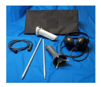
The Lmic is an easy-to-use, low cost, electronic listening stick and ground microphone combined. It is ideal for general leak sounding operations and can be fitted with either a tripod foot (for use as a ground microphone) or probe rods (for sounding at fittings or in soft ground).
