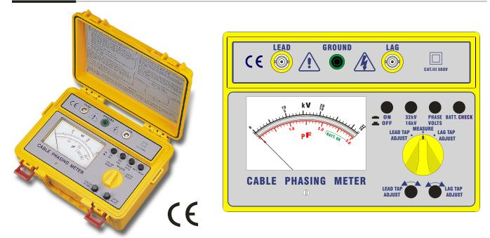
The **4183 CP** is a Cable Phasing Meter that offers a quick method of measuring voltage and determining phase rotation of underground distribution systems using the capacitive test point of elbow connectors. Most manufacturers of high voltage cable terminations incorporate capacitive test points in their elbow connectors. These test points are designed for measuring purposes.
